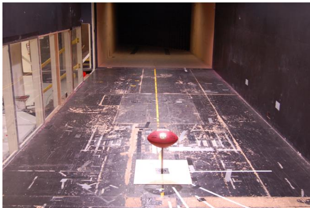
Fig 5. Experimental set up of NFL ball in the test section of RMIT Industrial Wind Tunnel at 90^\circ yaw
